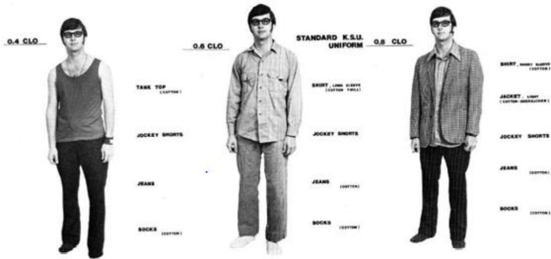
Figure 2.25: Clothes insulation diagram (1 clo = 0.155 \text{ m}^2 \text{ K} / \text{W} ), from Webdelson.com (2014)
