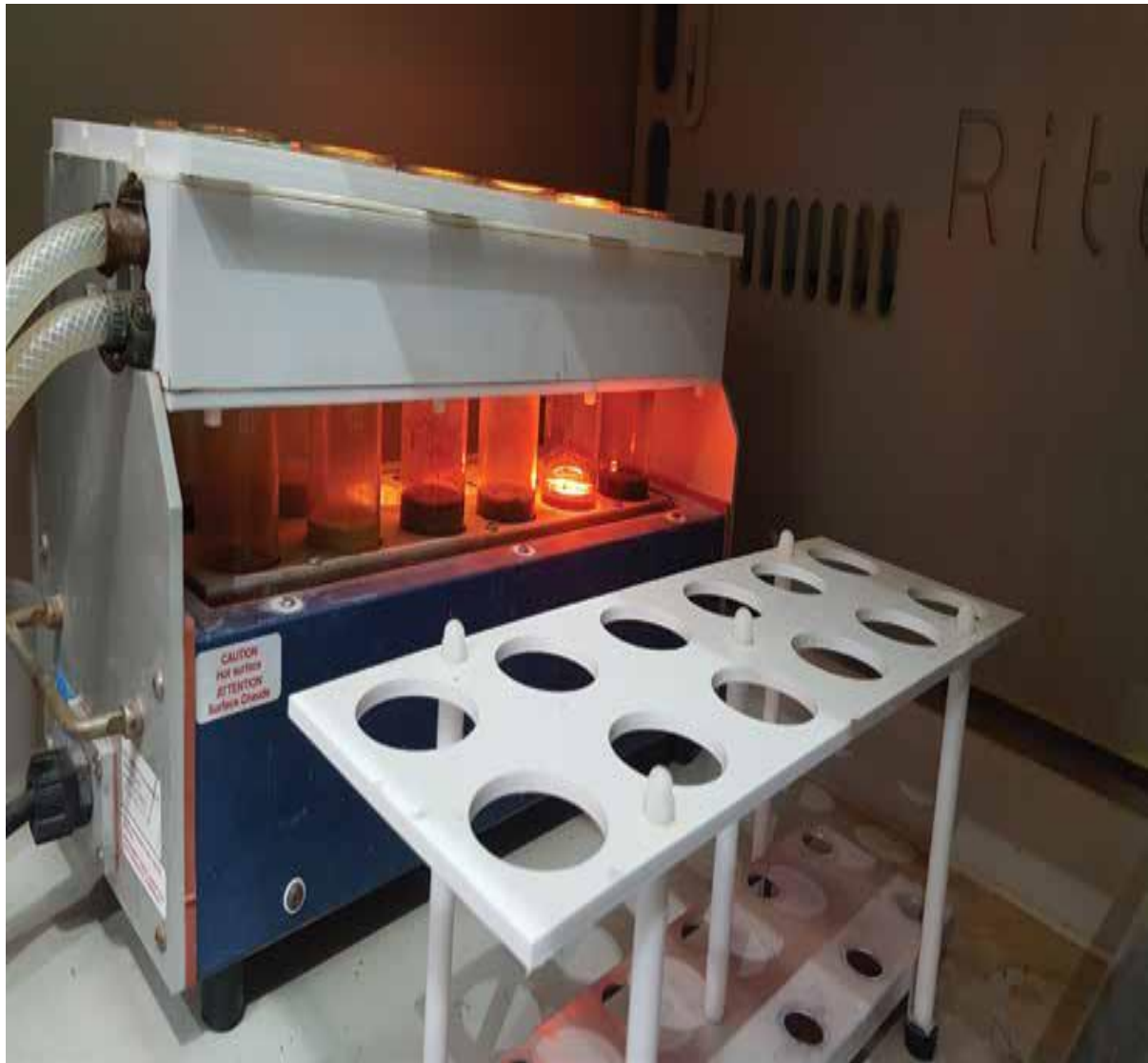
Figure 2.2: Coldblock Digestion Set Up
