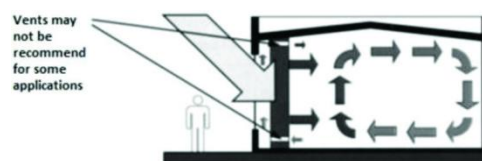
Figure 2.7: Indirect gain schematic. Source: (Izzet & Tulay, 01 July 2019)
