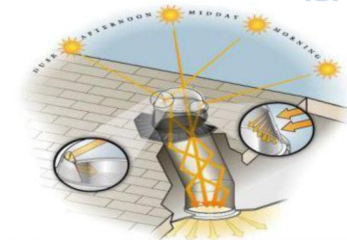
Figure 2:8 Showing Tubular Light
