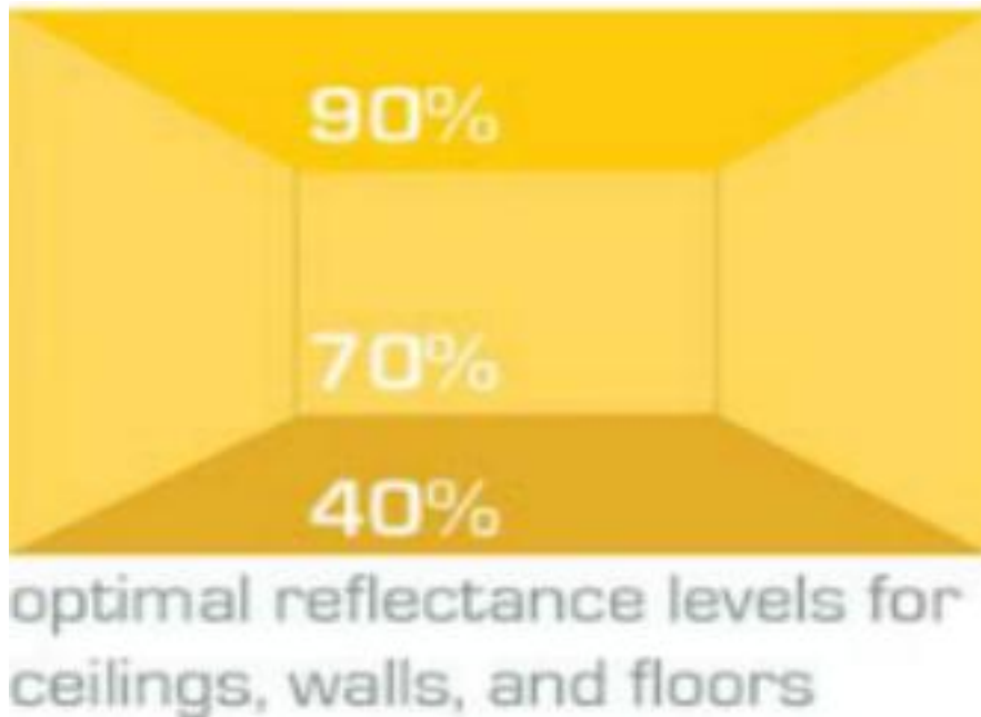
Figure 2.2 Showing Daylighting Principles Source: (Ashraf & Abdin, 2024).
