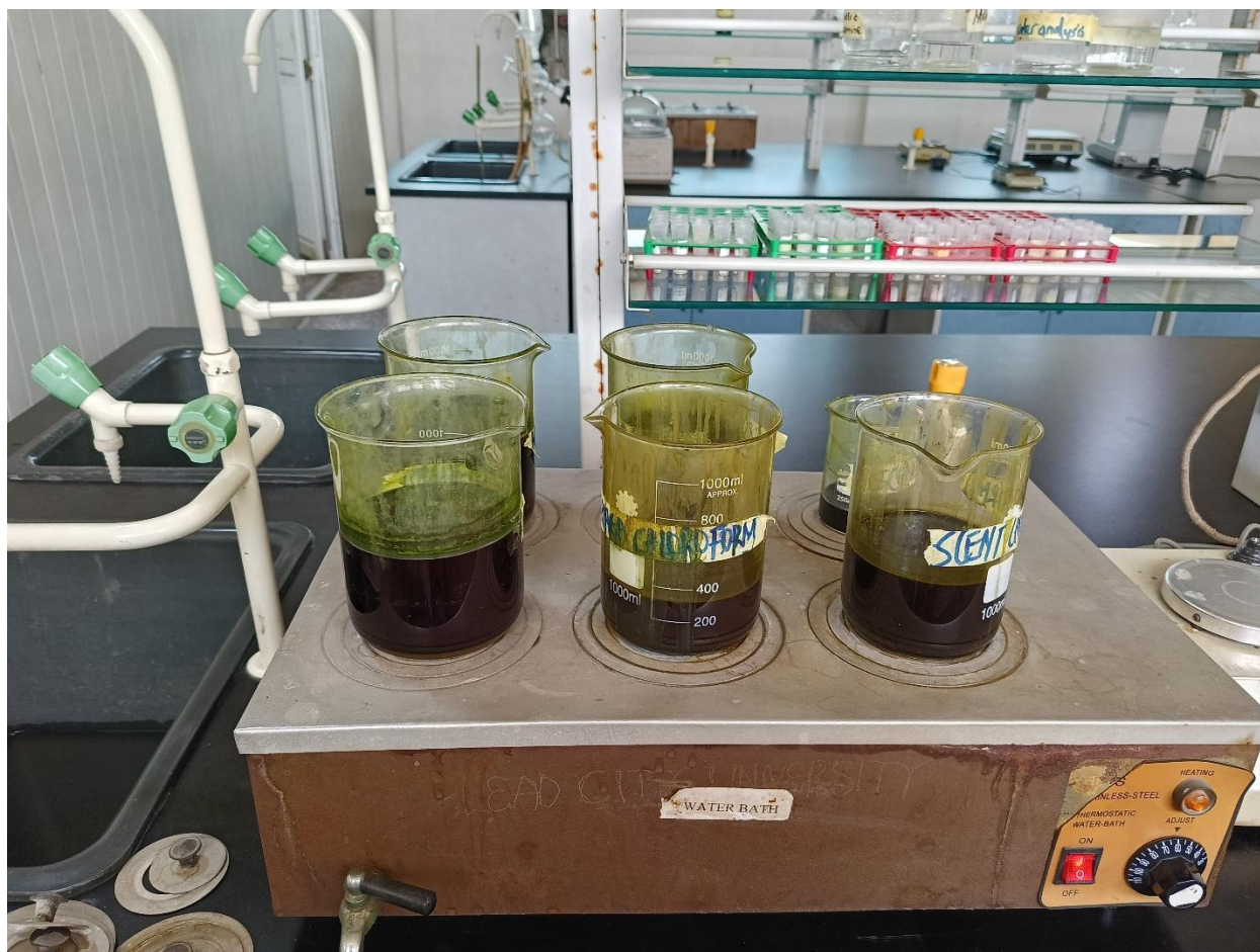
Extraction process of Ocimum gratissimum and Moringa oleifera leaves
