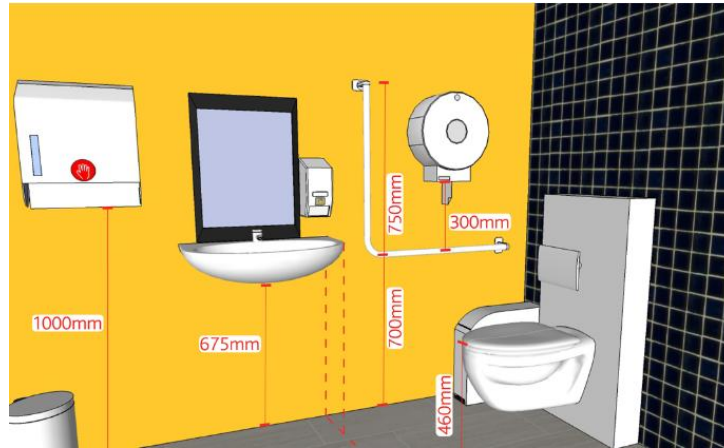
Plate 4.51: Showing Accessible Toilet
