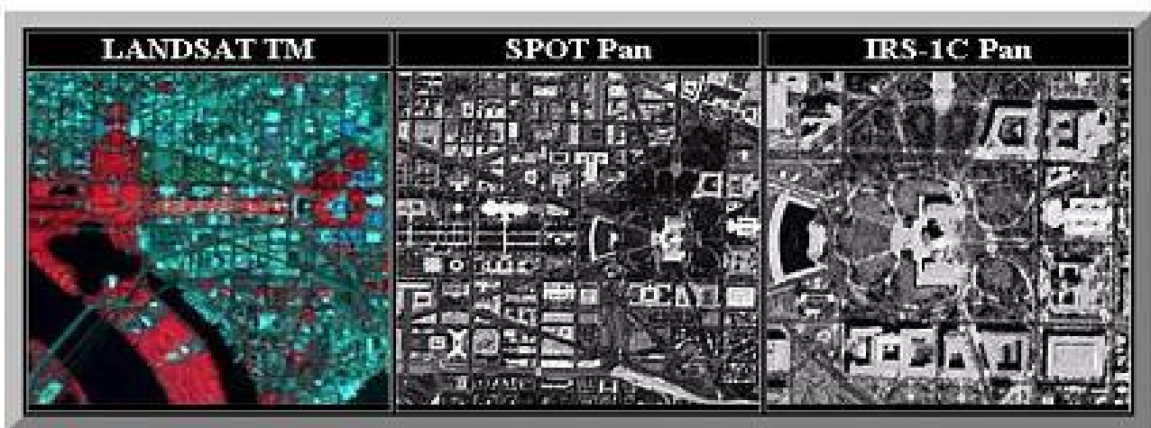
Figure 2.7: Illustration of Satellite Imageries Resolution
