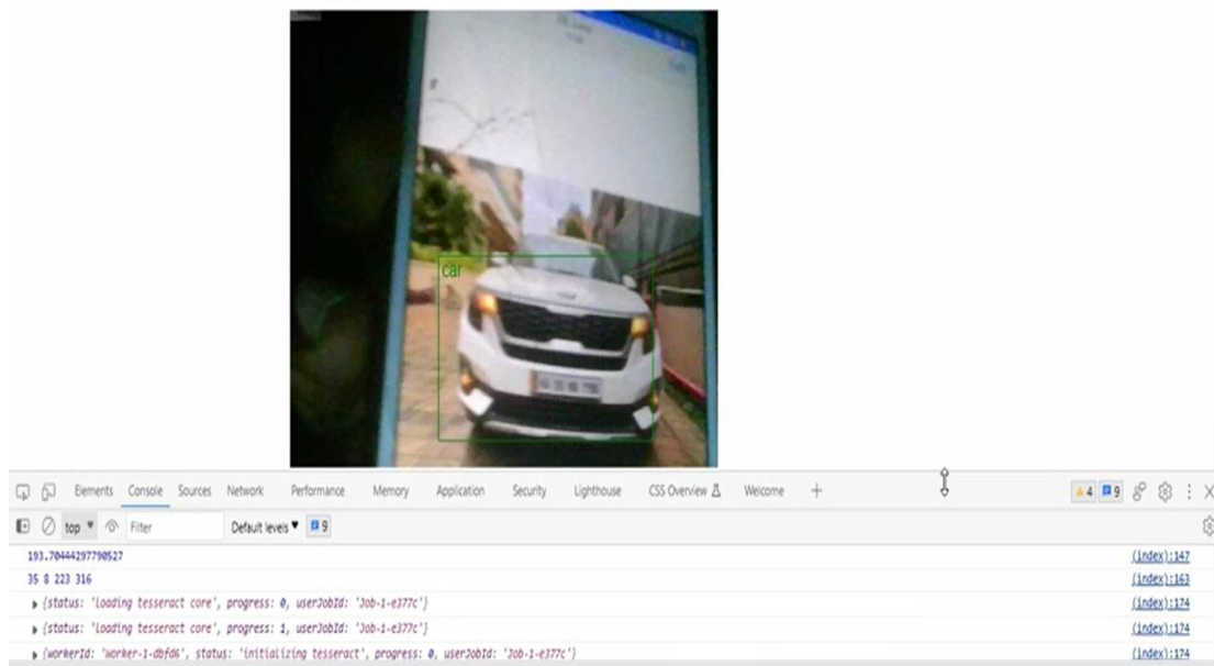
Figure 4.9: Display of Car Plate Number Showing x, y Position, Width And Height
