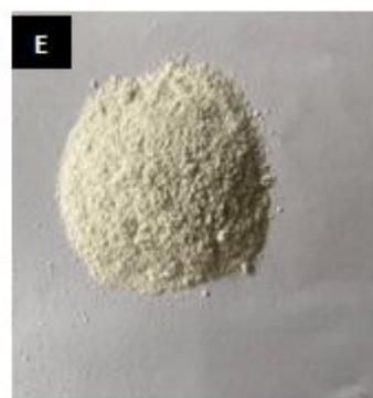
Figure 4.3: Nanocatalyst samples: (A) SS (B) SS powder (C) calcined SS (D) SS doped with Aluminum Chloride hydrated and Ferric Chloride (E) SS doped with Aluminum chloride hydrated
