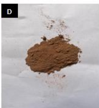
Figure 4.3: Nanocatalyst samples: (A) SS (B) SS powder (C) calcined SS (D) SS doped with Aluminum Chloride hydrated and Ferric Chloride (E) SS doped with Aluminum chloride hydrated
