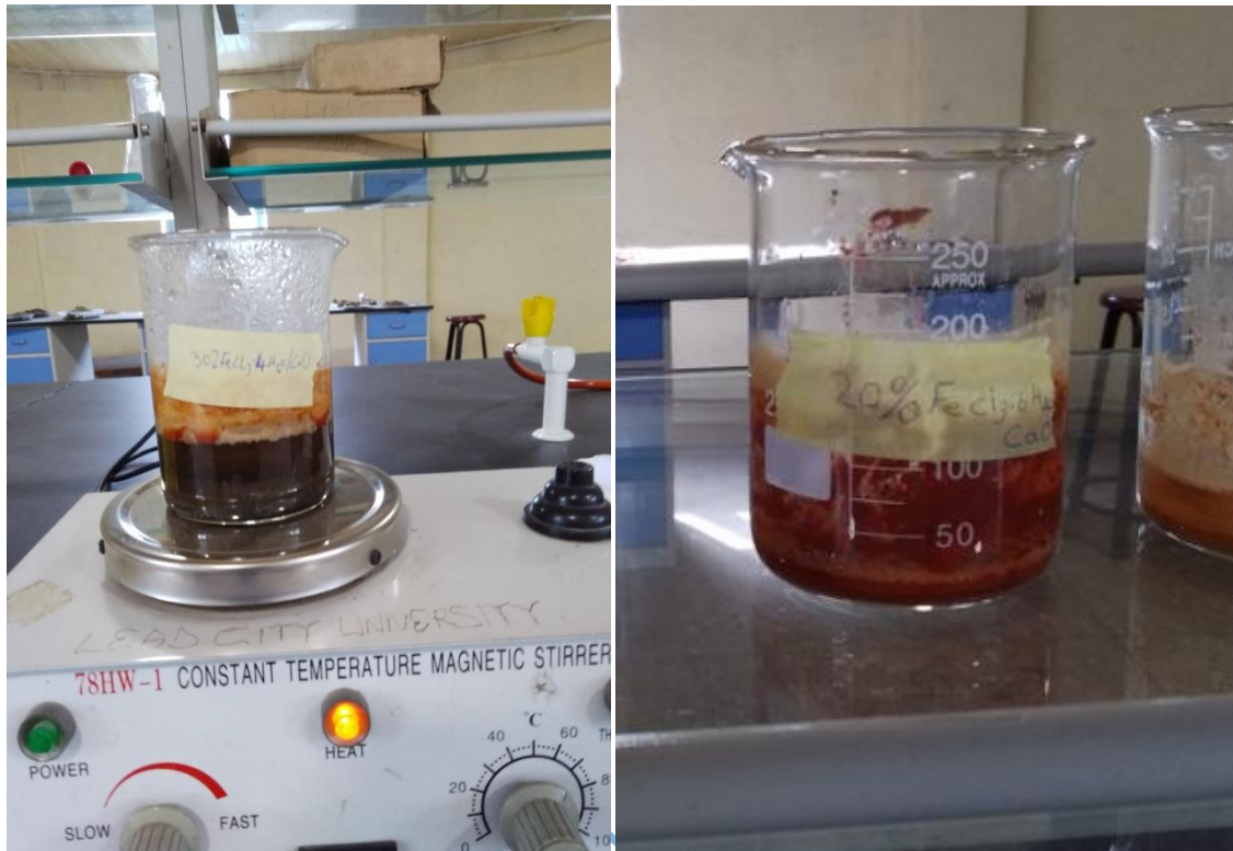
Figure 4.1: Preparation of SS doped with Ferric chloride by wet impregnation.
