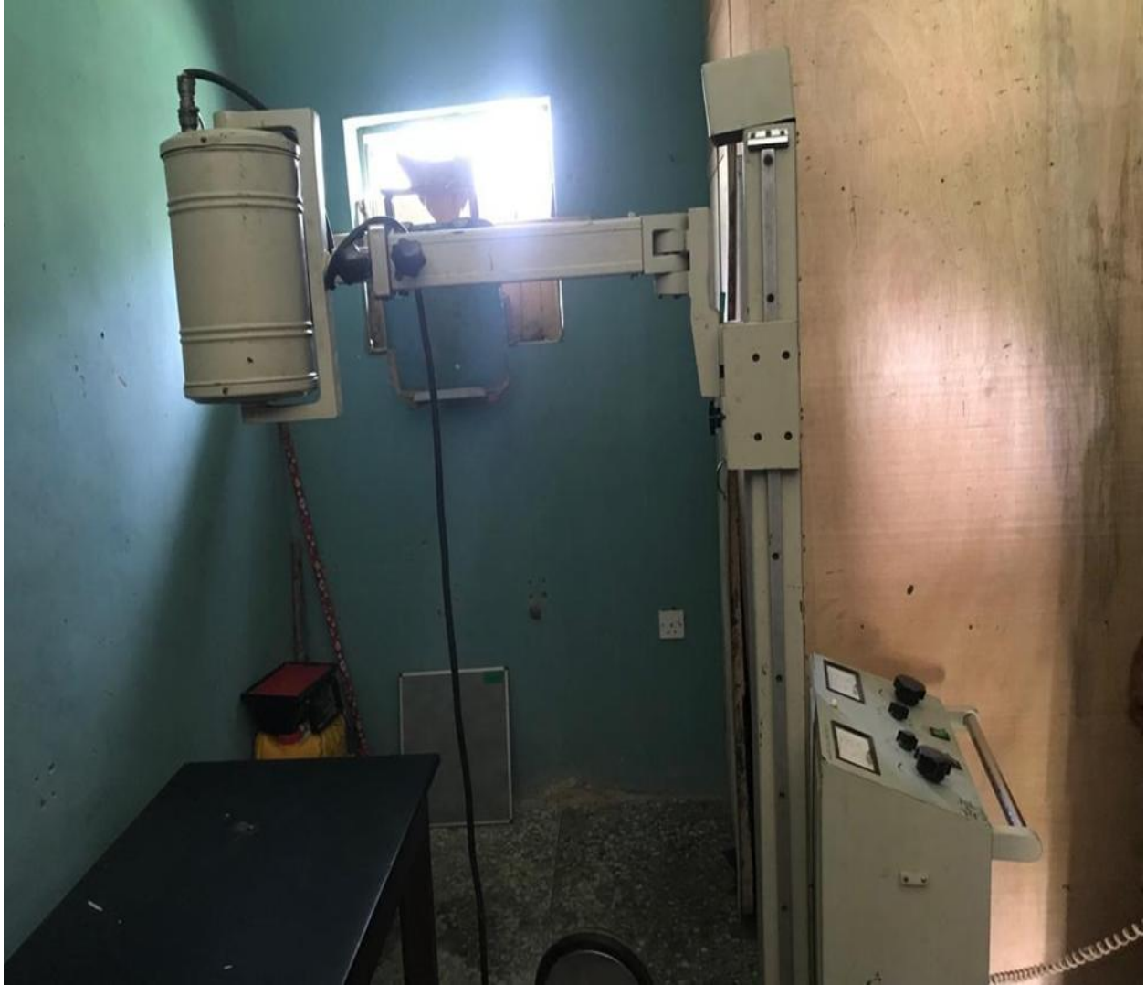
Figure 3.13: Picture from Centre H, no sign of radiation protection was seen in this facility.
