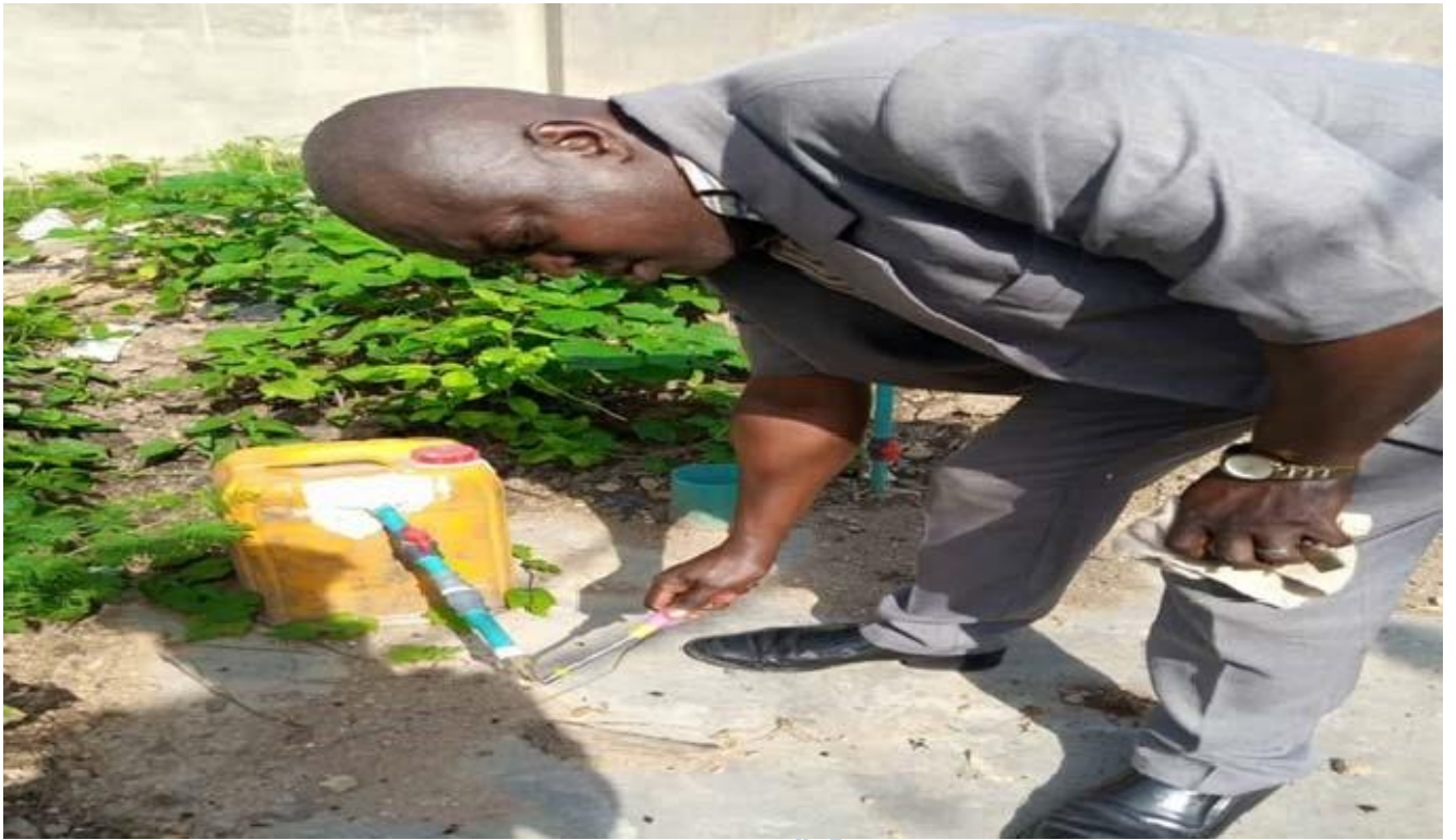
Plate 4.3: Researcher testing the flame coming out of the methane chamber with lighter
