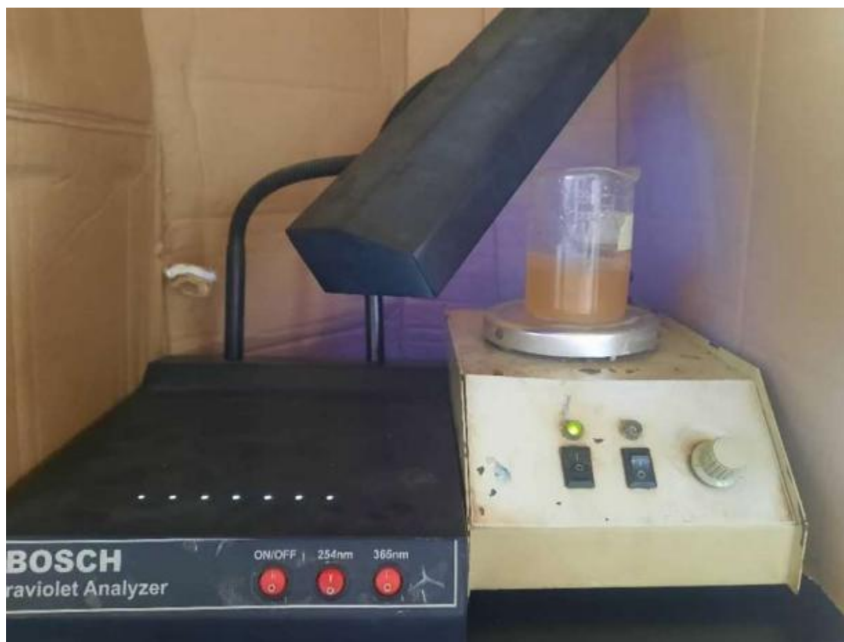
Figure 3.6: Photocatalytic degradation of antibiotics using UV-light
