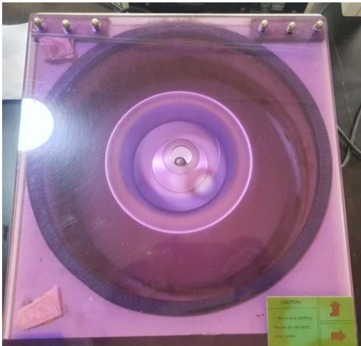
Figure 3.7: Centrifuging reaction after photodegradation to extract the biosynthesized nanoparticles.
