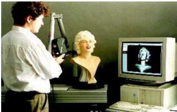
Figure 2, Manually operated arm and strip 3D scanner
