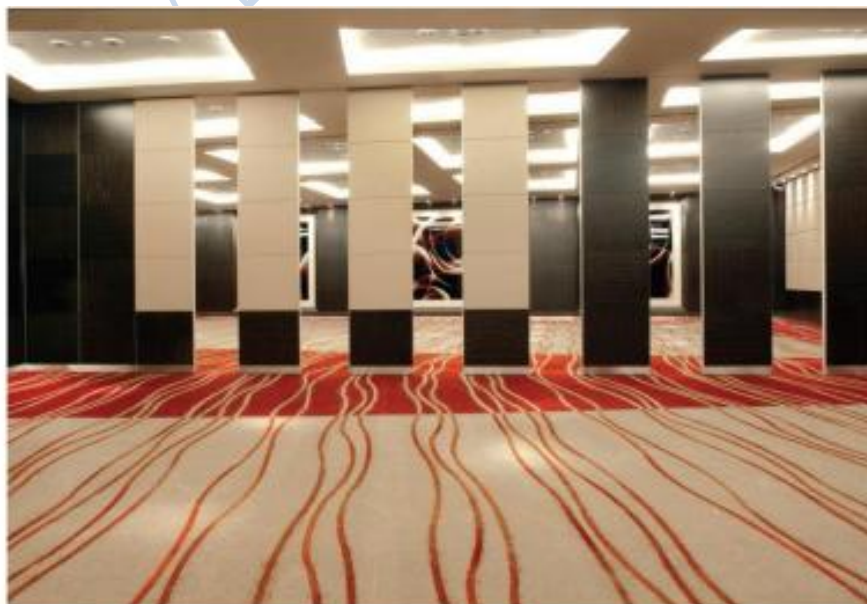
Figure 8: Sliding Wall System (Accordial)
