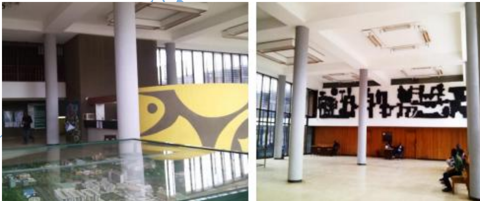
PLATE 10: Double volume space for reception, general waiting, and exhibition with 600mm diameter columns spaced @ 7m c/c (Source – Author's field work)
