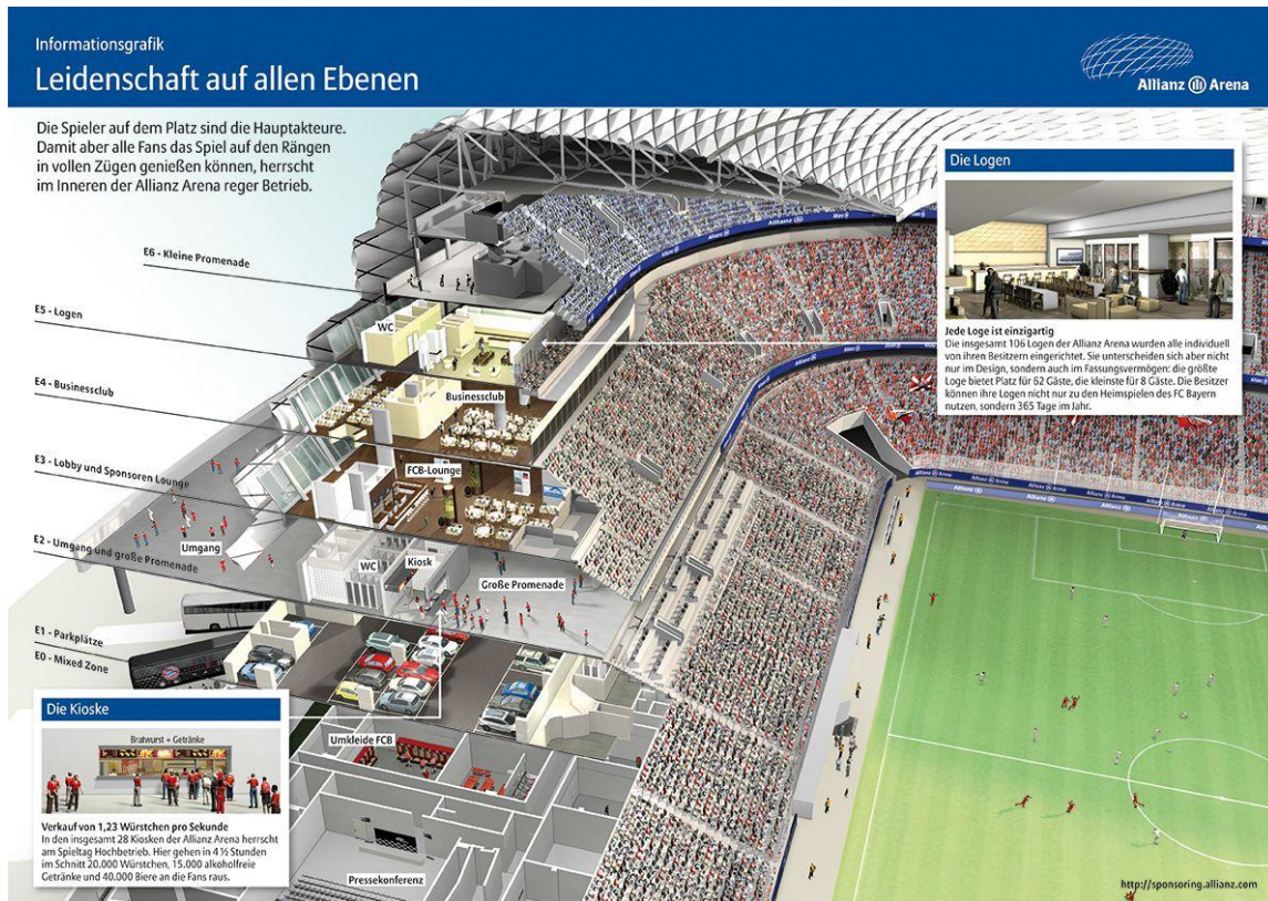
Fig 3.5: Section Through the Stadium Building.
