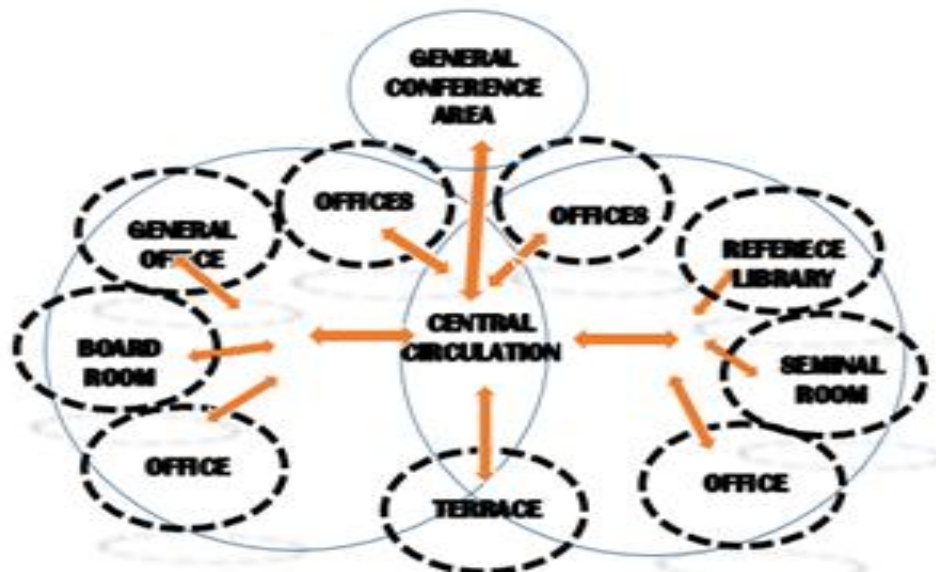
Figure 4.7 Bubble Diagram of showing Functional relationship (second floor) Source: Author's Field survey.
