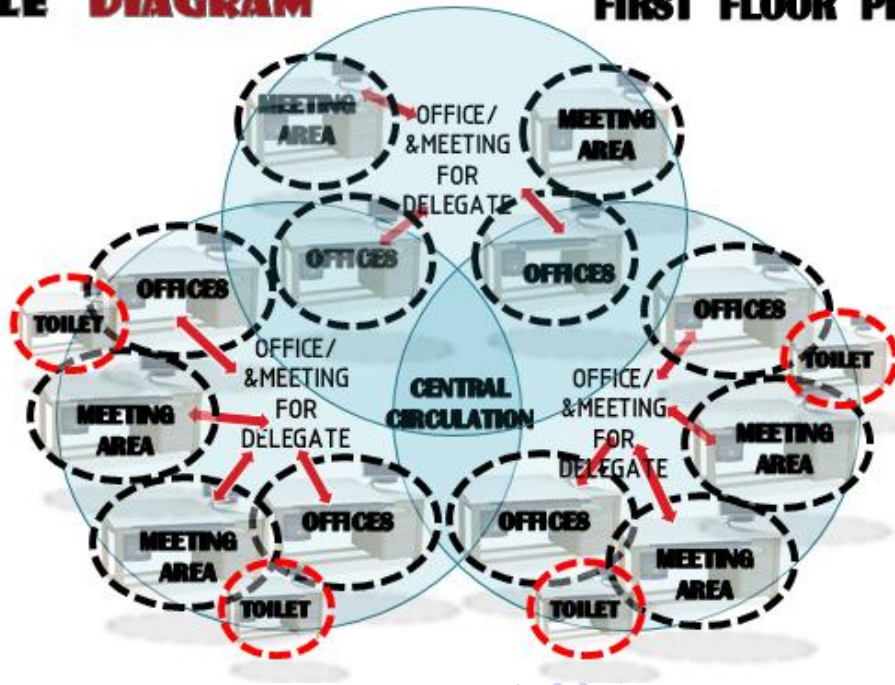
Figure 4.6 Bubble Diagram of showing Functional relationship (1st floor plan) Source: Author's Field survey.
