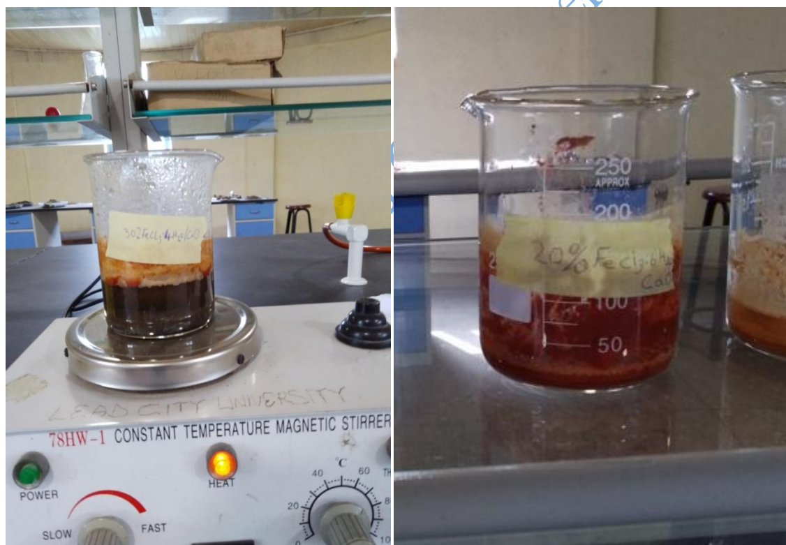
Figure 4.1: Preparation of snail shell doped with ferric chloride by wet impregnation
